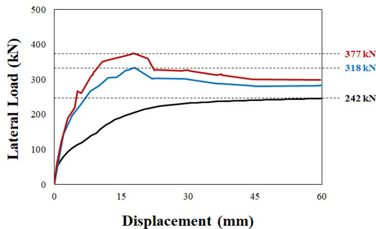
**Fig. 2** Load-Displacement Relationship of Diaphragm and Slab Model
